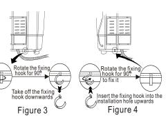
Drain hose fixing hook
